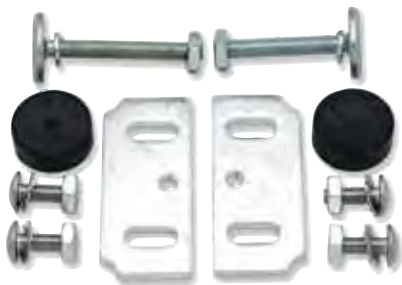
INSIDE TOP WINDOW STOP SET These mount inside the door at the top and act as a stop for the window and allow for adjustment to the upward travel. One set required per door. Hardtop and convertible only, will not work on sedans. 1955-57 Hardtop & Convertible.... #2193..... $27.95/set
